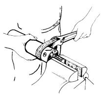
Remove all fittings, rotate barrel counterclockwise with a strap wrench one full turn. Locking wire will feed out of slot during turning. At the completion of revolution, remove retaining wire, wiggle barrel and slide from head.
